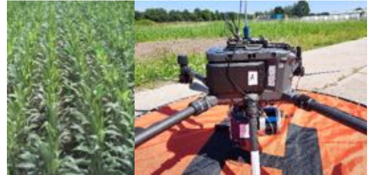
Headwall Nano-Hyperspec VNIR Spectral range: 400 – 1000 nm 270 spectral bands
