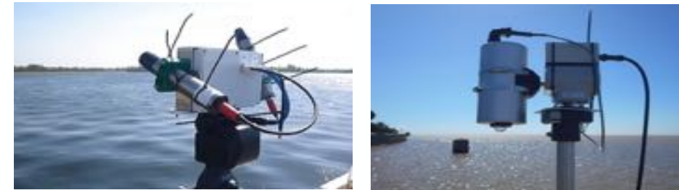
(PANTHYR radiometer System and HYPSTAR® radiometer system. Cable tie spikes are used for bird avoidance)
