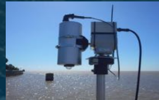
(PANTHYR radiometer System and HYPSTAR® radiometer system. Cable tie spikes are used for bird avoidance)
