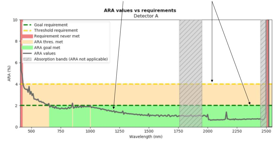
Absolute Radiometric Accuracy (%) against requirements, instrument is here simulated as « End-of-Life » (i.e. « worst-case »).
